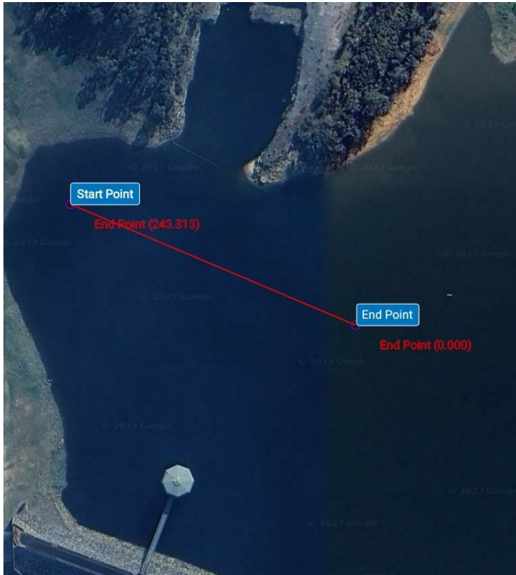
Figure 4 Transect line of the dam floor survey, used for this risk assessment.
